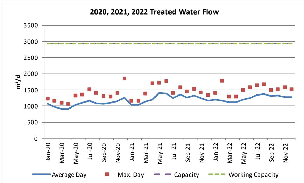
Maximum treated water demand was observed in February 2022. The cause is due to a large commercial fire on the MBQ. During 2022, there were zero service leak repairs, one hydrant repair and one watermain break repair. A six inch watermain was installed and into service in May 2022 to service a 10 plex on the North end of Green Street.
